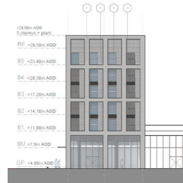
Fig 7.74 SH8 North Elevation
