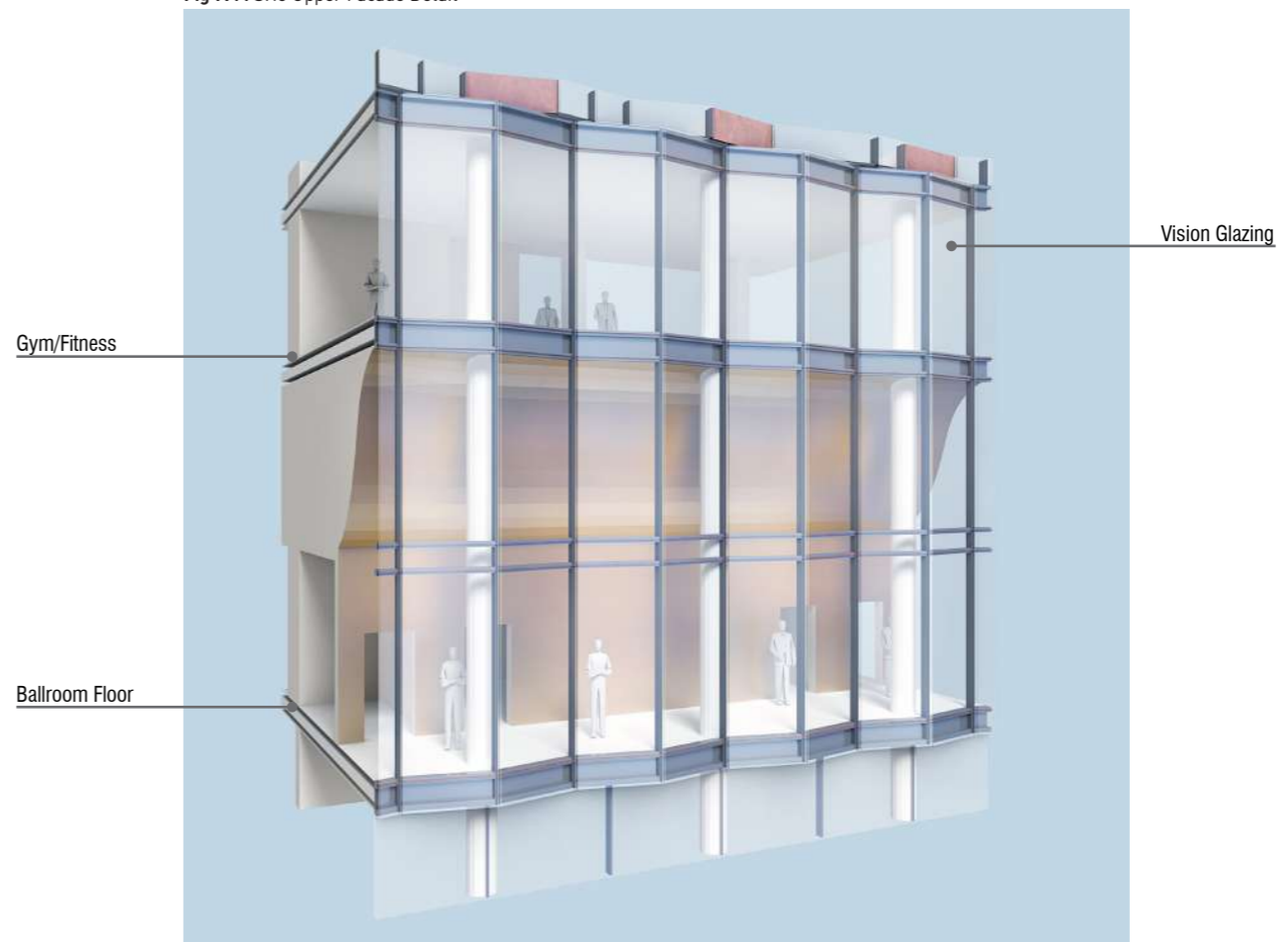
Fig 7.45 SH5 Lower Facade Detail
