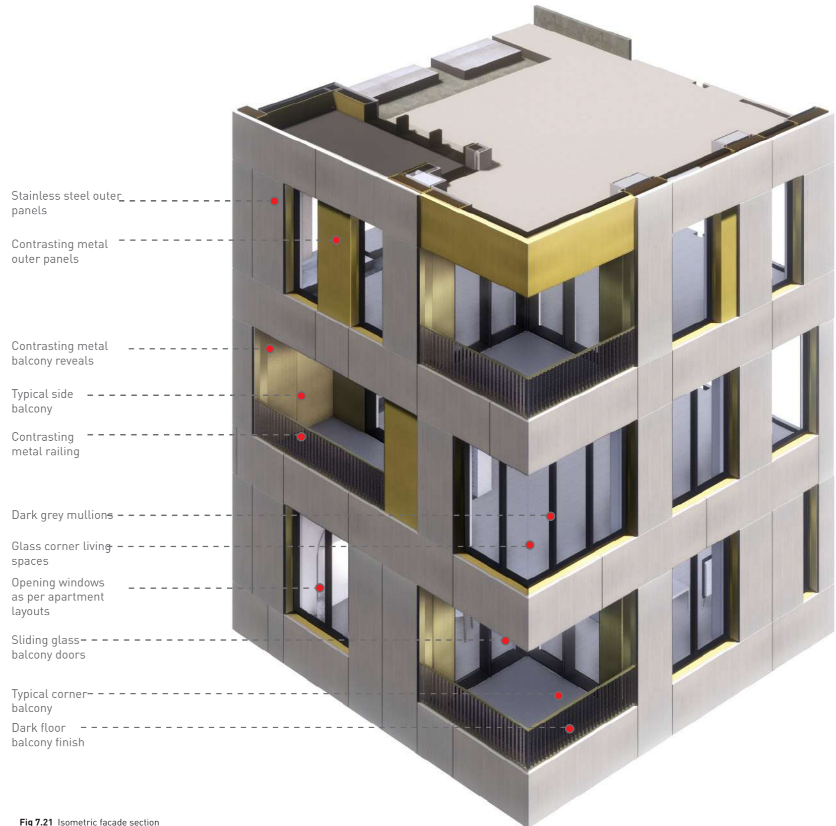
Fig 7.21 Isometric facade section
